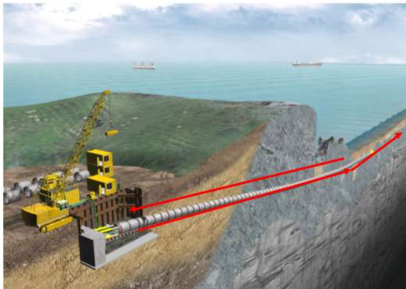
Figure 1: Simplified image of the process of microtunneling: the technology allows to introduce the pipeline below the seabed, in order to discharge far from the coasts without the use of ships.
