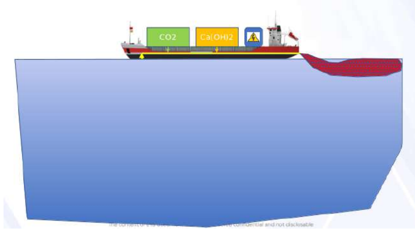
Figure 2: Schematic representation of the surface discharge process: the ship is equipped with containers of CO_2 and Ca(OH)_2 to buffer the bicarbonate solution in order to discharge water with the same pH as the draft water.
