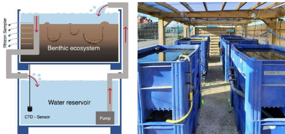
Figure 3. In the benthic mesocosms at the University of Antwerp the dissolution kinetics of silicate minerals and the impacts on the benthic fauna in coastal environments have been monitored since 2019. The system comprises 20 units with two stacked tanks: the upper tank houses the benthic ecosystem, and the lower tank functions as a water reservoir. Natural sediment of 40 sediment heights with a mean grain size of 123\ \mu\text{m} ( 3.0\ \phi ) was collected from an intertidal sand flat in the Oosterschelde (the Netherlands) and mixed with olivine sand of similar grain size. Water from the Eastern Scheldt Estuary (salinity 32–35) is used to conduct flux sessions of 5 weeks (weekly sampling). At the end of each session, the total volume of water in each unit ( \sim 500\ \text{L} ) is renewed (drawing: Astrid Hylén (UAnt); photo: Matthias Kreuzburg, https://www.coastal-carbon.eu/ , last access: 7 November 2023, Geobiology, University of Antwerp).
