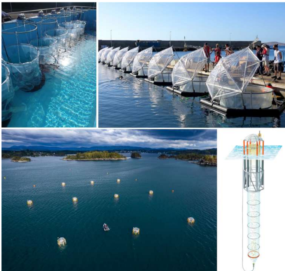
Figure 1. Pelagic mesocosm facilities currently used in OAE research. Top left: land-based mesocosms ( 1\text{ m}^3 ) at the University of Vigo, Spain. Top right: in situ on-shore mesocosms ( 10\text{ m}^3 ) operated by GEOMAR, here employed on Gran Canaria, Spain. Bottom left: Kiel Off-Shore Mesocosms for Ocean Simulations (KOSMOS), here employed in the Raunefjord, Norway. Bottom right: sketch of a KOSMOS mesocosm unit ( 55\text{ m}^3 ). Image sources: (top left) Daniela Basso, University of Milano-Bicocca; (top right) Ulf Riebesell, GEOMAR; (bottom left) Uli Kunz; (bottom right) Rita Erven, GEOMAR.
